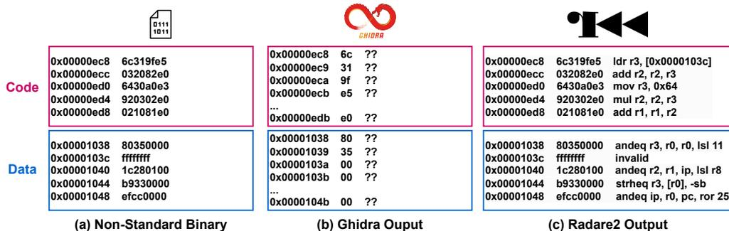
Figure 1: Outputs of Ghidra and Radare2 when a non-standard binary is used as the input. We use red and blue to indicate the ground-truth code and data. Ghidra does not load the non-standard binary correctly, and Radare2 treats everything as code to perform linear sweep. Neither can separate data from code.
